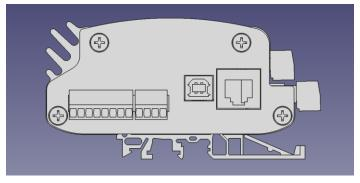
Clearance required for right side connector. Insure clearance is provided for airflow around heat sink fins when operating at higher current levels. Avoid mounting controller inverted as this traps air in the heat sink fins. Insure clearance on left side for wiring, USB, and Ethernet connectors.
